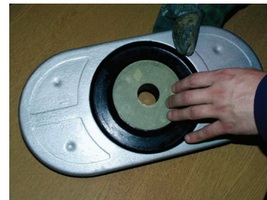
Gentle press seal to ensure cohesion
